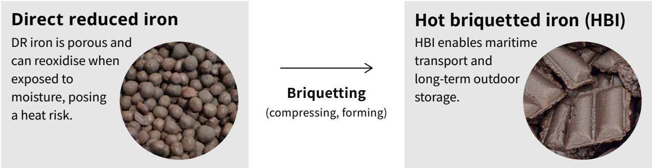
Figure 12: Direct reduced iron and hot briquetted iron
